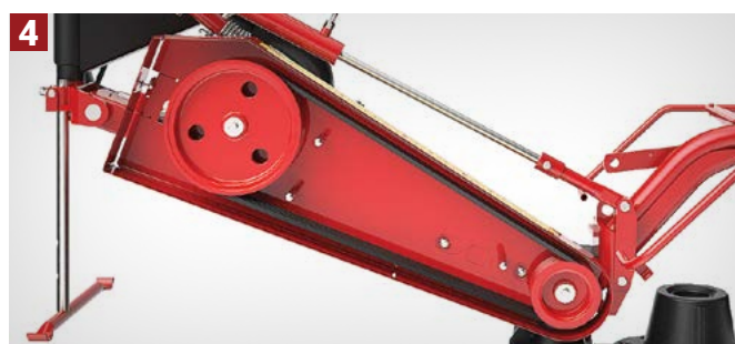
A SET OF V-BELTS transmits power to gearbox.
