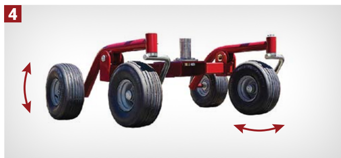
4 WHEELS OPTION: VERTICAL WHEEL MOVEMENT by \pm 10^\circ improves ground contour adaptation. Turning the first pair of wheels allows the tractor to change direction without lifting the machine.
