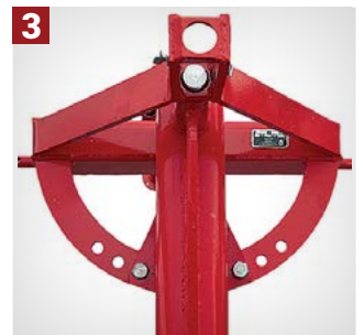
SNOWPLOUGH MOUNTING BRACKET: Horizontal angular adjustment of snowplough, and possibility of 360 degree rotation
