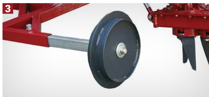
THE WORKING DEPTH is adjustable with a 2-wheel frame
