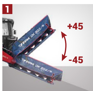
WORKING POSITION Designed to work on slopes from -45 up to +45 degrees.
