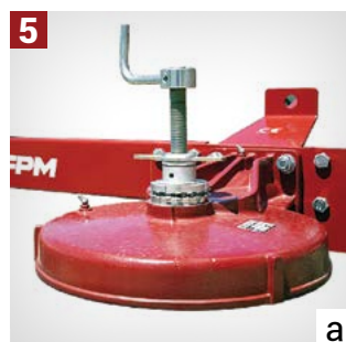
WORKING HEIGHT ADJUSTMENT: a) by adjusting gearbox height; b) by adjusting wheel height.
