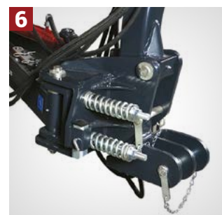
PROTECTIVE MECHANISM with springs, allows the current displacement of the side mulcher in a collision with an obstacle
