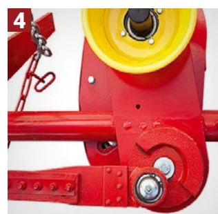
FRAME: Safety system for automatic release of the cutter bar in case of obstacle impact;
