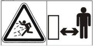
Rotating elements! During the machine's operation, there is a possibility of objects being thrown from the ground at a great distance. Keep a safe distance from the machine.
