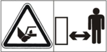
Rotating elements! Keep a safe distance from the machine's moving parts while the tractor is in operation, and the Cardan joint is turned on.
